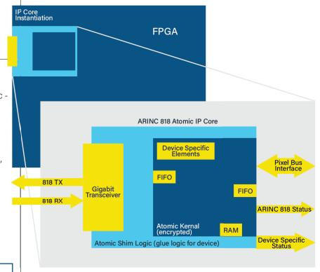
FEATURES: The ARINC 818 Atomic IP Core is compile-time configurable to match the specific requirements of your ARINC 818 video format. Features and supported formats include:
